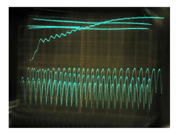
I powered on my R390-A's using my variac to produce 200V at C606A with 3 different 0A2's and they regulated correctly. I scoped the voltage and again saw no voltage above 200V during warm up.
